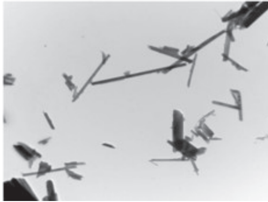
Fig. 2. TEM image of \text{Li}_2\text{B}_4\text{O}_7:\text{Cu} sample exposed to 5 \times 10^{11} ions/cm 2 \text{Ag}^{9+} beam
